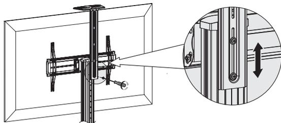
Attach the connecting plate to the column at the desired height using the appropriate screws. Tighten all screws using a suitable screwdriver.
